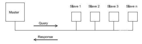
In the MODBUS Protocol the master can address individual slaves, or, using a special "Broadcast" address, can initiate a broadcast message to all slaves. The power sensor do not support the broadcast address.
