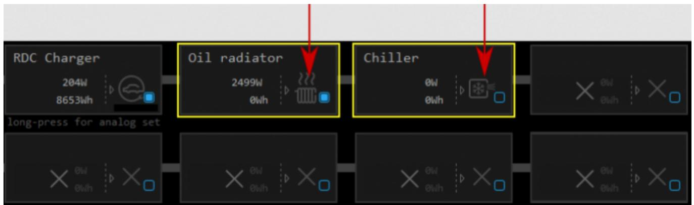
**Note:** Nominal power **P nominal** is suitable for consumer(s) without connected power sensor. It is used for consumed energy calculation during active mode.
