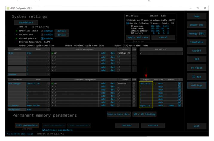
HEMS Configurator → settings → enter name and select icon (2). Message "Error - device is not responding" may appear as IP address is not defined yet.
