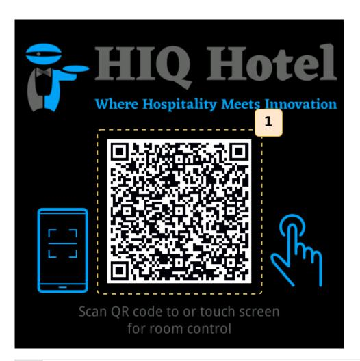
QR code link for the mobile GUI web page. To manage the room, scan the code with a smartphone. The website address and QR code automatically change when a new guest checks into the room, preventing former guests from controlling the room.
