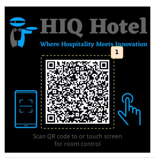
**1** QR code link for the mobile GUI web page. To manage the room, scan the code with a smartphone. The website address and QR code automatically change when a new guest checks into the room, preventing former guests from controlling the room.
