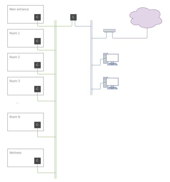
Each access point has its own unique identification (AP\_ID), assigned by the system integrator during system setup.
